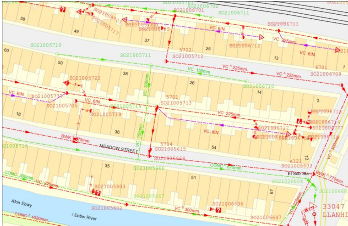
Figure 4: Plan showing the drainage infrastructure of Meadow Street and Railway Street (DCWW, 2020)
